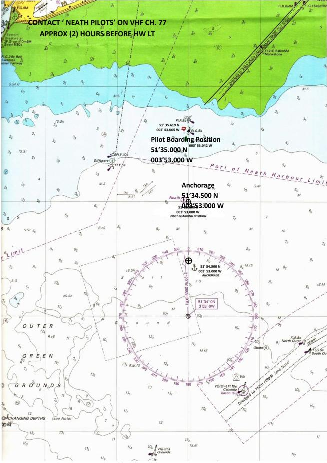
VESSEL TO BE UNDERWAY **(2) HOURS BEFORE HW** – PILOT WILL BOARD AT THE PILOT BOARDING POSITION APPROXIMATELY **(1) Hr (40) Min BEFORE HW.** CONTACT 'NEATH PILOTS' VHF CH. 77, FURTHER INSTRUCTIONS ON COURSE,SPEED & BOARDING SIDE WILL BE GIVEN. PILOT LADDER RIGGED TO 2M ABOVE THE WATER.
